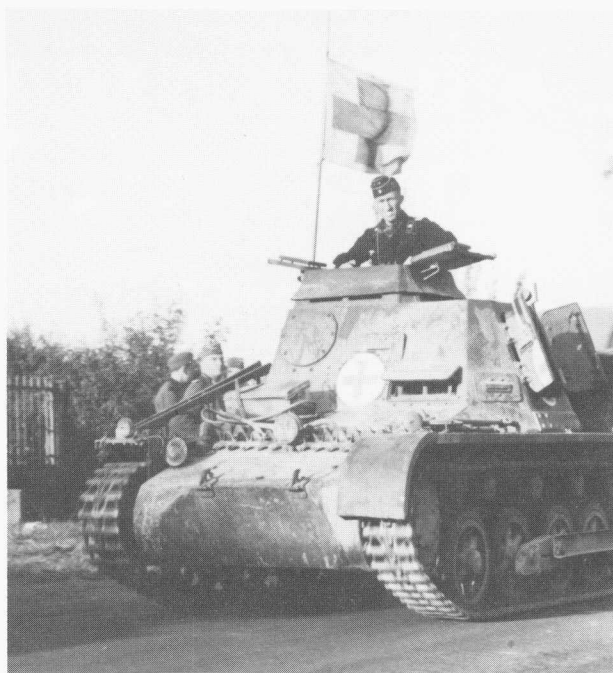
Kleiner Panzerbefehlswagen of 4.Pz-Div. used as an ambulance vehicle in France, 1940; note red cross markings on front and sides, and divisional insignia just visible above the visor. Other ambulance conversions of the PzKpfw I had cut-down, open-topped superstructure. (US Nat. Archives)
