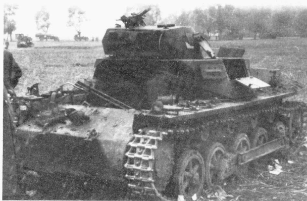
The PzKpfw I's armour was barely sufficient to protect it from machine gun fire. (Above), a tank with the hull front completely caved in by a direct hit from a Polish 75mm field gun during September 1939: 53 of the 89 PzKpfw Is lost in Poland were total combat losses. (via Steven Zaloga) (Right), a PzKpfw I Ausf. B of 4. Pz-Div. in France, 1940, also completely destroyed by an artillery hit. (US Nat. Archives)
